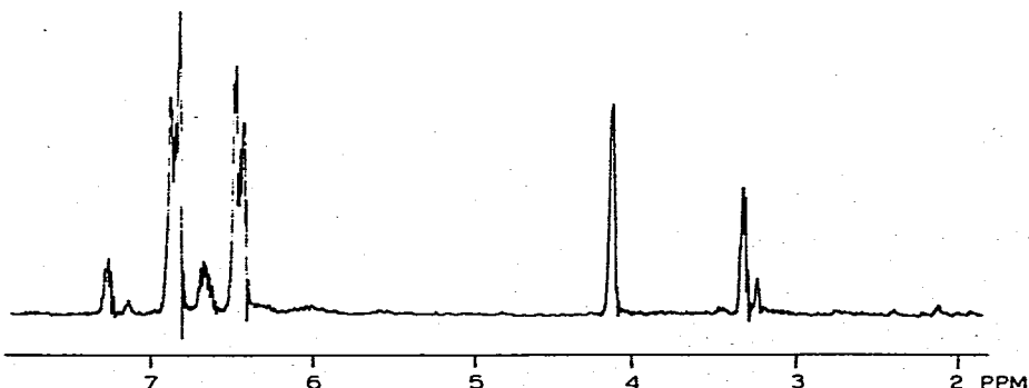
Fig. 1. 100 MHz PMR spectrum of II in \text{CS}_2 at -52^\circ\text{C} .
